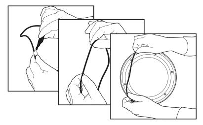
Figure 4. Installing the O-Ring
